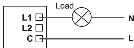
**Figure 2.** Using a 1 or 2-Way Dimmerswitch
