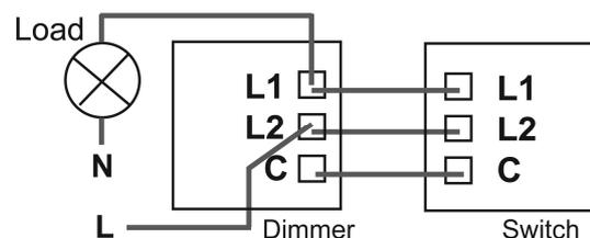
**Figure 4.** Using a 2-Way Dimmerswitch
