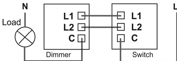
**Figure 3.** Using a 2-Way Dimmerswitch
