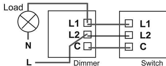
**Figure 4.** Using a 2-Way Dimmerswitch
